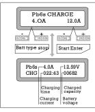
Set up the charge current on the left and the nominal voltage of the battery on the right. The charge current ranges from 0.1 to 5.0A. and the voltage should match with the battery being charged. Start the charge process by pressing start The screen displays the state of charging process. To stop charging forcibly, press batt type stop key once. The audible sound indicates you the end of
