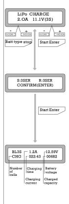
The value on the left side of second line sets a charge current and the value on the right side of second line sets the voltage of the battery pack. After setting the current and voltage press start enter key for more than 3 seconds to start the process. (Charge current: 0.1--5.0A, Voltage: 1---5 series)
